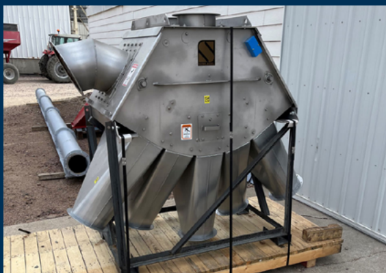
This stainless-steel distributor, with heavy-duty plastic liner, was installed in the coop's east feed mill early in November. It will reduce feed hang-up and risk of cross-contamination.
